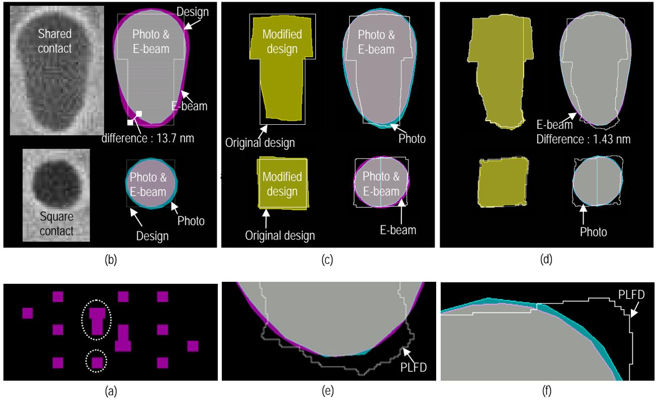
Fig. 8. PLFD results of contact patterns in 65-nm node scale SRAM cell: (a) the original CP-cell; (b) EBL resist pattern images of shared contact and square contact patterns, and those contour images by EBL and photolithography simulations; (c) first modified pattern results; (d) final modified pattern results (e) the enlarged picture at the bottom of the shared contact in (d); (f) the enlarged picture at the upper right of the square contact in (d).
