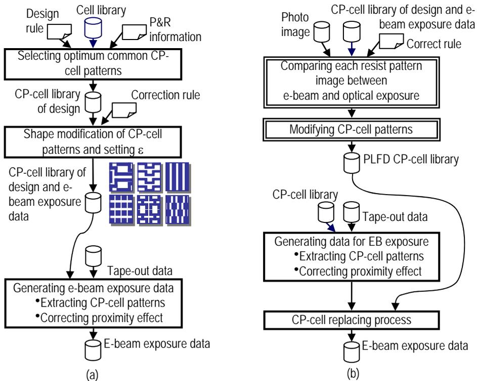
Fig. 6. Data processing flowcharts: (a) the conventional flowchart for CP exposure data; (b) the new flowchart for applying PLFD CP exposure data.
