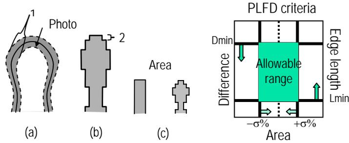
Fig. 5. Criteria for applying PLFD CP-cells and the allowable range: (a) The difference from photo image is labeled “1”; (b) The edge length is labeled “2”; (c) The irradiate area difference in a PLFD CP-cell and the original CP-cell.
