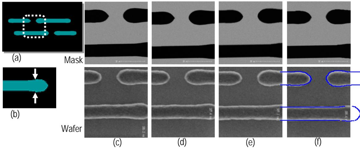
Fig. 12. Dependence on the grid size: (a) the PLFD CP-cell data by the 0.1 nm contour grid size; (b) the measurement point; (c) SEM images on mask and on wafer by the 0.1 nm contour grid; (d) SEM images on mask and on wafer by the 1.0 nm contour grid; (e) SEM images on mask and on wafer by the 2.0 nm contour grid; (f) SEM images on mask and on wafer by the 1.0 nm contour grid, and is overlaid with the target contour of the photolithography.
