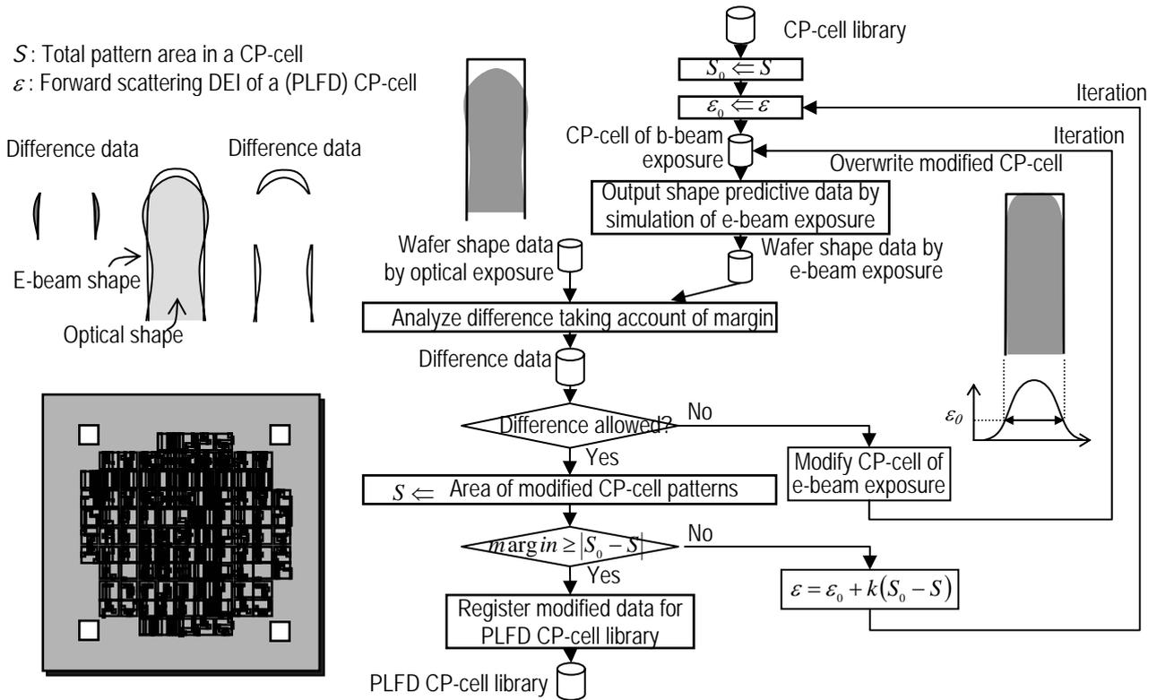
Fig. 7. Flowchart of the process creation PLFD CP-cell library for the e-beam exposure.
