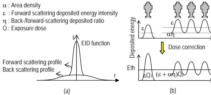
Fig. 4. Schematic diagram of the correction concept for PLFD. (a) The forward scattering effects are corrected using pattern shape modification; and the backscattering effects, using dose correction. (b) The backscattering effects to a PLFD CP-cell are corrected with its dose correction only.
