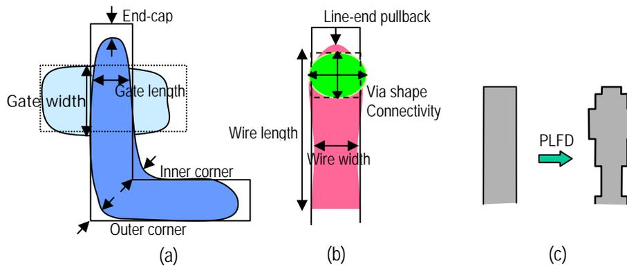
Fig. 2. Printability problems and Photolithography-friendly design. (a) Transistor shape has effects on transistor characteristics;  $V_{th}$ ,  $I_{on}$ , and  $I_{off}$ . (b) Wire shape has effects on wire characteristics; Capacitance, Resistance, Via resistance, and Dielectric. (c) Schematic illustration of PLFD
