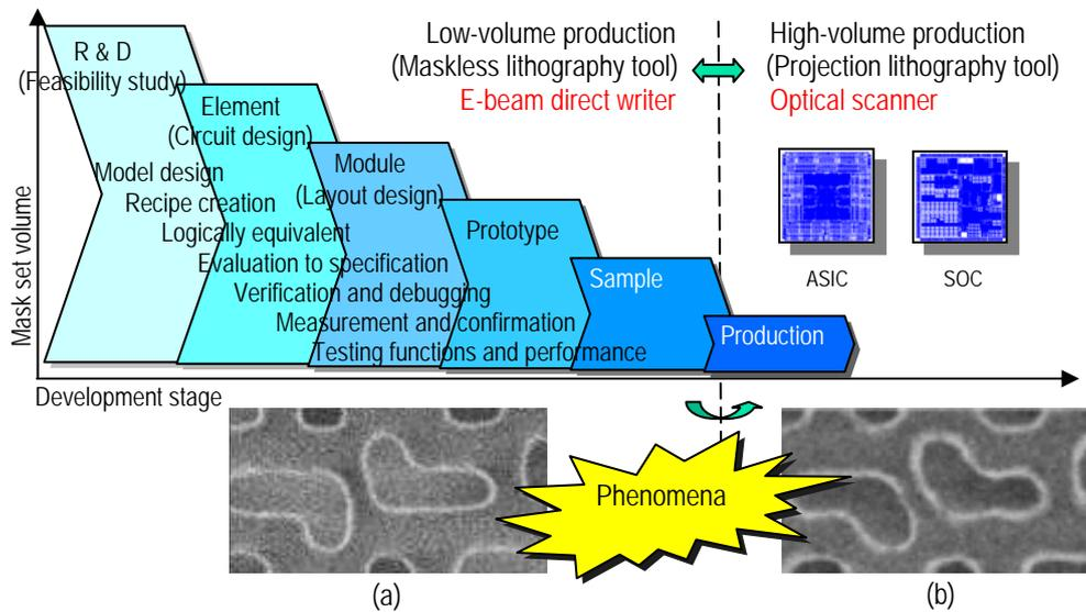
Fig. 1. Relation between device development stages and lithography tools, and comparison of the shape of resist patterns between electron beam and ArF exposure: (a) SEM image by electron beam exposure; (b) SEM image by ArF.
