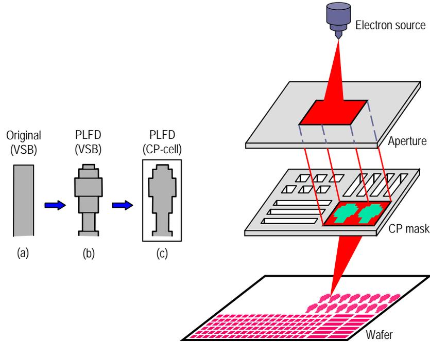
Fig. 3. Schematic representation of an e-beam cell projection (CP) exposure method. (a) The shot count of this original pattern is one with various shaped beam (VSB). (b) The shot count of the PLFD pattern is 6 with VSB. (c) The shot count of the PLFD pattern is one with CP.
