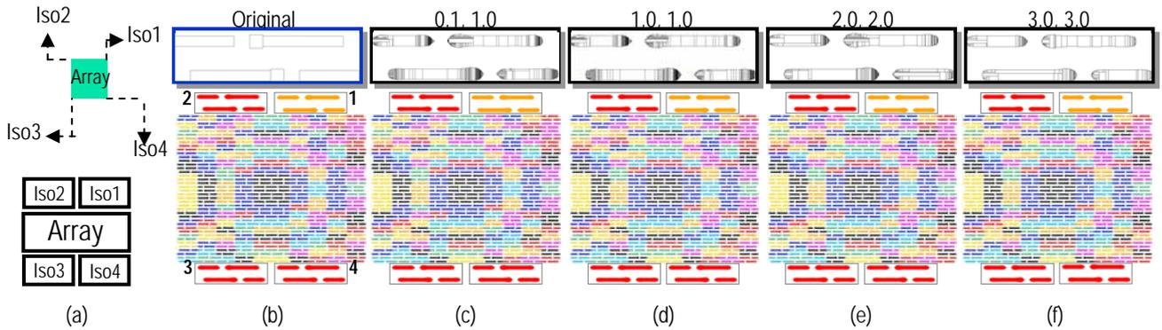
Fig. 10. Relationship between the contour grid size and the exposure dose: (a) geometry of CP-cell; (b) original CP-cell; (c) PLFD CP-cell by 0.1 nm contour grid and 1.0 nm modify grid; (d) PLFD CP-cell by 1.0 nm grid size; (e) PLFD CP-cell by 2.0 nm grid size; (f) PLFD CP-cell by 3.0 nm grid size.
