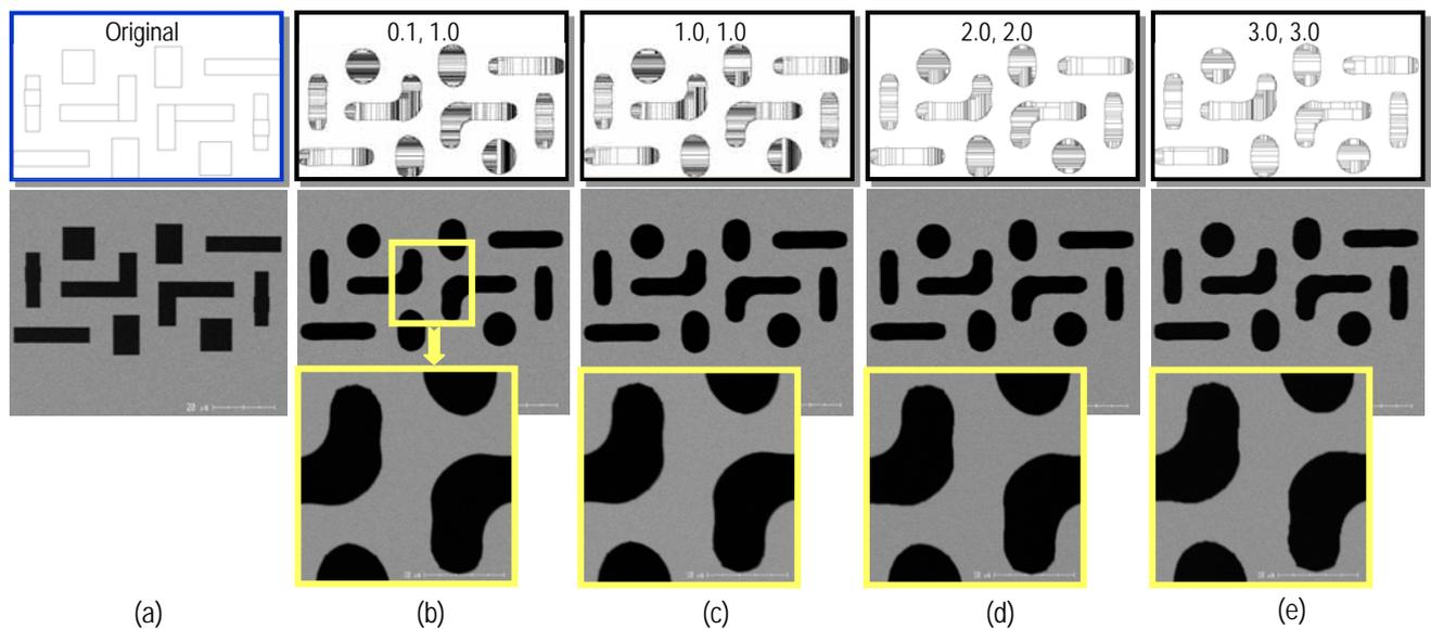
Fig. 9. Relationship between the contour grid size and CP mask: (a) the original CP-cell; (b) PLFD CP-cell by a contour grid size of 0.1 nm and a modify grid size of 1.0 nm; (c) PLFD CP-cell by the contour of 1.0 nm and the modify of 1.0 nm grid size; (d) PLFD CP-cell by 2.0 nm grid sizes respectively; (e) PLFD CP-cell by 3.0 nm grid sizes respectively.
