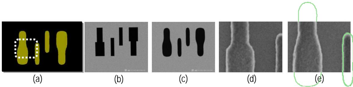
Fig. 11. SEM images on mask and on wafer: (a) the PLFD CP-cell data by the 0.1 nm contour grid size; (b) the original CP-cell on mask; (c) (a) on mask; (d) a portion on wafer exposed with (b); (e) a portion of the square in (a) on wafer, and is overlaid with the target contour of the photolithography.
