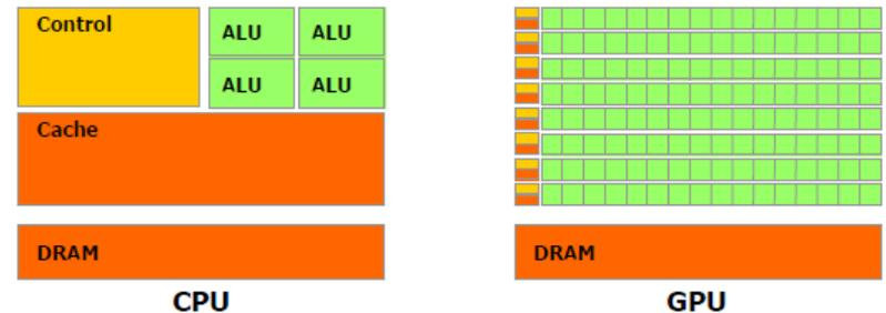
Architecture of CPU and GPU
