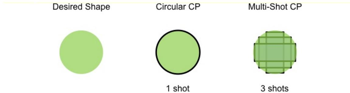
*Figure 4. Overlapping several rectilinear shots to create one “multi-shot” CP enables circular CP for machines without the ability to include circles on stencils.*
