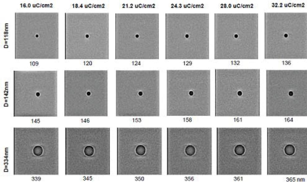
Figure 11. Resist-exposed images of the circles with various doses.
