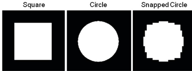
Figure 5. Layout used in the simulation. The contacts are all on a 200nm by 200nm pitch. The square pattern is 120nm by 120nm in size, the circle radius was set to 67nm and the shape of the snapped circle were adjusted in order to get approximately the same maximum intensity for all three contacts. Note that to match the area of the square, the circle diameter would need to be equal to 67.7nm which is quite close to the value used to match the maximum intensity.
