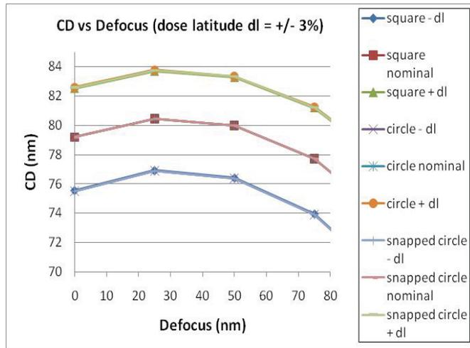
Figure 8. CD versus defocus for nominal dose, nominal dose – dl (dose latitude), nominal dose + dl for all three contact types. The dose latitude dl was set to 3% of nominal dose. Very small adjustments of the threshold to get the same CD of 80nm for all three contacts made the curves perfectly overlay.
