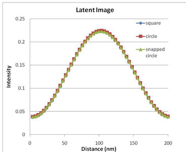
Figure 6. Latent image for the circle, square, and snapped circle.
