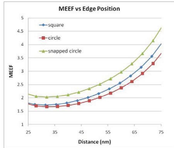
Figure 9. MEEF versus edge position for square, circle, snapped circle.
