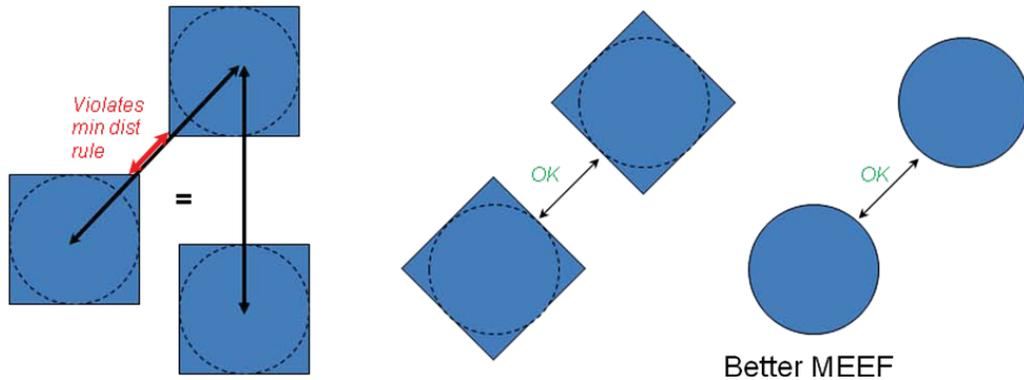
Figure 1. Vias and contacts on masks drawn as circles reduce the Mask Error Enhancement Factor (MEEF).
