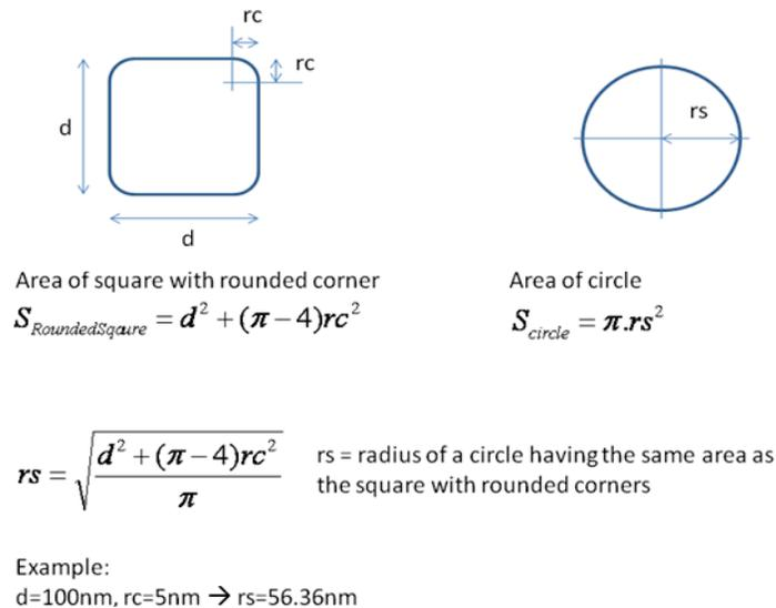
Figure 2. Calculating the areas of rounded squares vs. circles. The radius of the circle  $rs$  is calculated to match the area of the square with rounded corners. All dimensions are at 1X.
