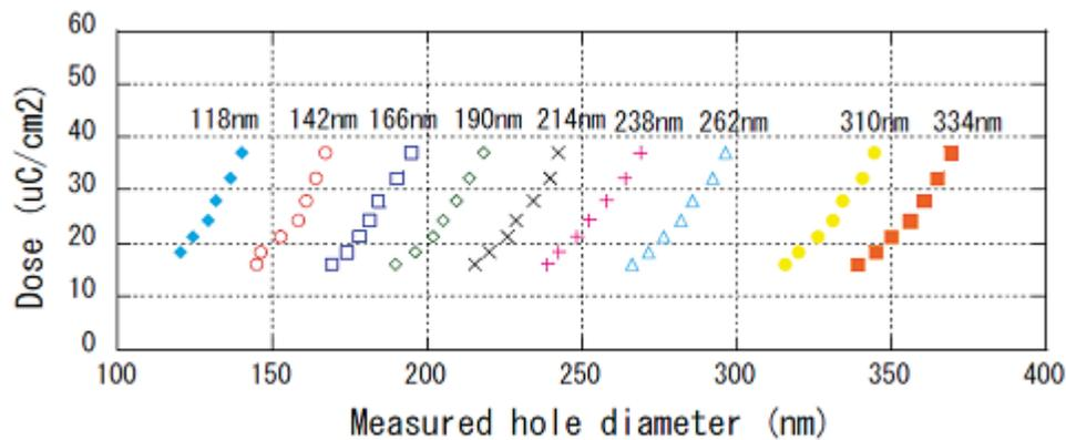
Figure 12. Measured diameters for each circular character as dose is varied.
