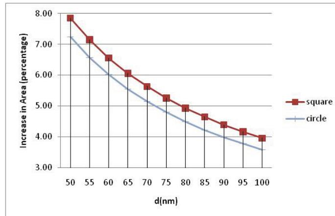
Figure 4. Increase in area for a rounded square and a circle of same area when the edge moves 1nm. All dimensions are at 1X.
