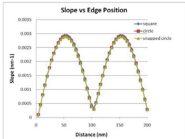
Figure 7. Slope versus edge position for the square, circle, and snapped circle.
