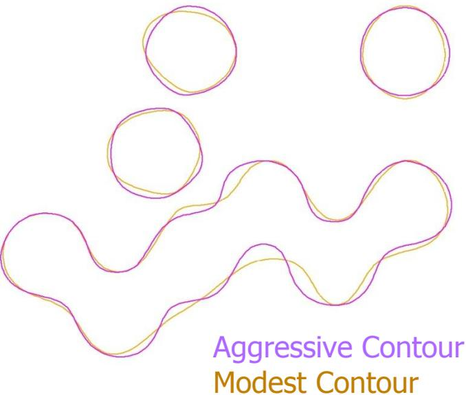
For coarser masks printing image degrades and can cause failure of guiding pattern to control positions of DSA cylinders
