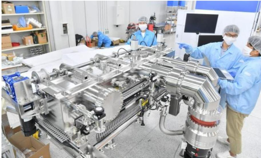
Researchers are manufacturing the main chamber part of the EUV light source in the clean room at ESOL, an EUV equipment company located in Dongtan Industrial Complex, Hwaseong-si, Gyeonggi-do.
