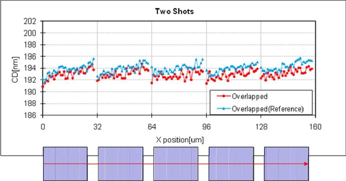
Figure 2. Measured CDs of line-space patterns L:S = 1:3, showing heat accumulation in each subfield.
