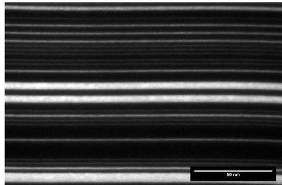
TEM images of the test pattern with linewidths down to 1.5 nm. The width of the lines was designed to form a pseudo-random test pattern; the pattern is used to characterize metrological instrumentation. The scale bar on the right image is 50 nm.
