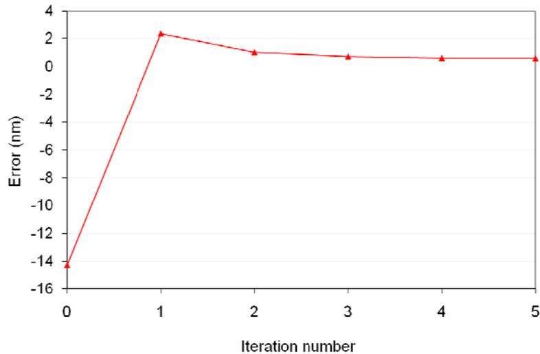
Figure 10. Proximity effect correction of large exposed pattern. This plot shows the edge position error in nanometer versus the iteration number.
