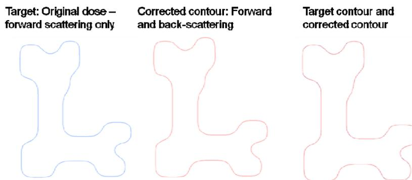
Figure 8. Left: contour with original dose and no back-scattering taken into account. Center: contour for the layout with corrected doses with forward and back-scattering taken into account. Right: Overlap of the contour in the center and the contour on the left.
