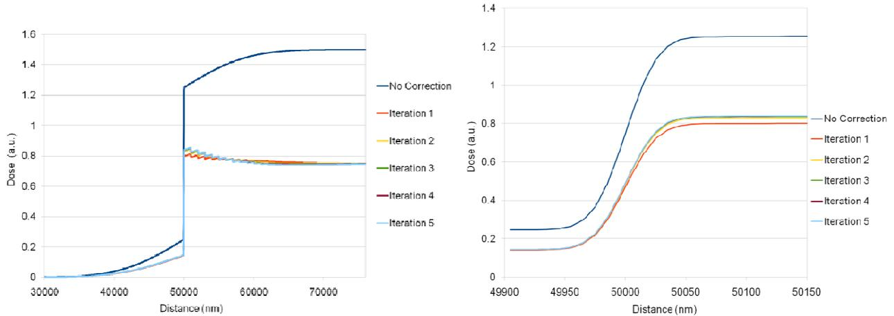
Figure 9. Dose versus distance for a 100 micron by 100 micron pattern on the right: before correction and after each iteration (from iteration number 1 to 5). The dose profile is computed taking into account forward and backscattering. The left plot gives an overview of the dose profiles; the right plot gives a closer look at the transition between the exposed and unexposed areas.
