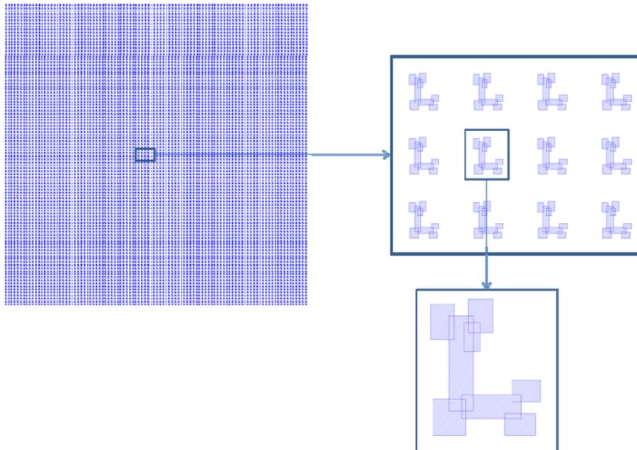
Figure 5. Test pattern comprising an array of "Ls". The picture on the left shows the entire layout. The pictures on the right show magnified views of the pattern. The pitch of the pattern in the x and y directions is 1 micron. The size of the entire pattern is 100 microns by 100 microns.
