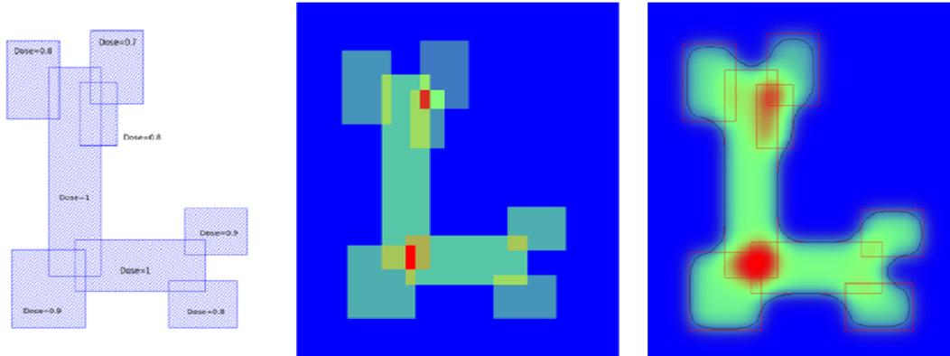
Figure 6. On the left, the pattern with the shots and the dose assigned to each shot. In the center is a dose map of shots. On the right is a simulation of the pattern taken into account only forward scattering. A contour at threshold 0.5 was overlapped in black.
