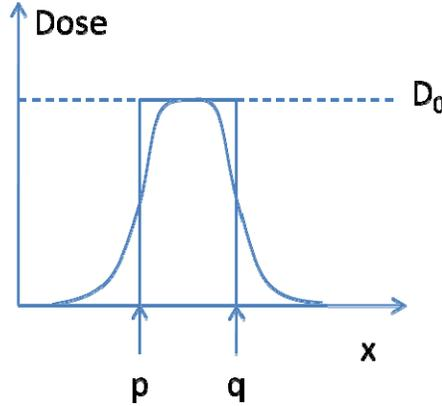
Figure 1. Forward scattering profile corresponding to a line exposed between location  $p$  and location  $q$  at a dose equal to  $D_0$ . The line is assumed to be infinite in the  $y$  direction.
