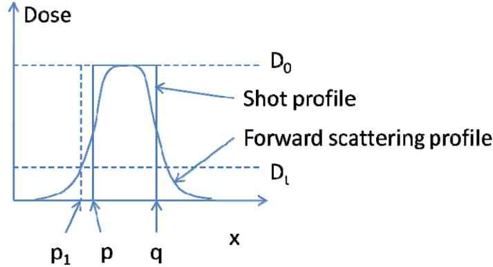
Figure 2. Forward scattering profile corresponding to a line exposed between location p and location q at a dose equal to  $D_0$ . The line is assumed to be infinite in the y direction. A dose threshold  $D_t$  is set to define the desired position of the mask edge  $p_1$ .
