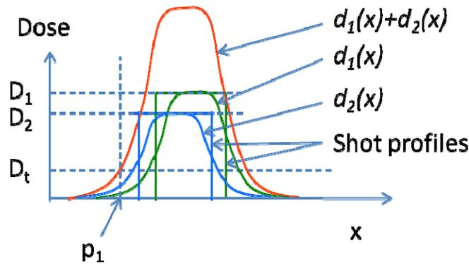
Figure 4. Forward scattering profiles for one exposure ( $d_1(x)$  and  $d_2(x)$ ) and for double exposure ( $d_1(x) + d_2(x)$ ) corresponding to an isolated line pattern. The line is assumed to be infinite in the y direction. The dose threshold  $D_t$  is set to define the desired position of the mask edge  $p_1$  for the combined exposure of the two shots.
