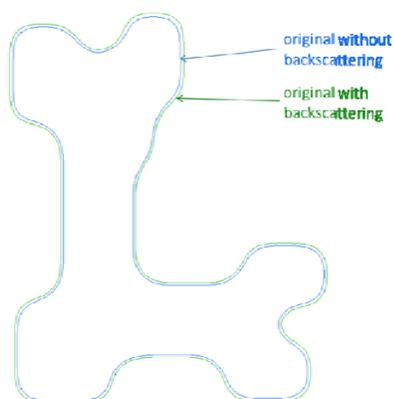
Figure 7. Contour without back-scattering taken into account and contour with back-scattering taken into account. No correction was applied to the shots.
