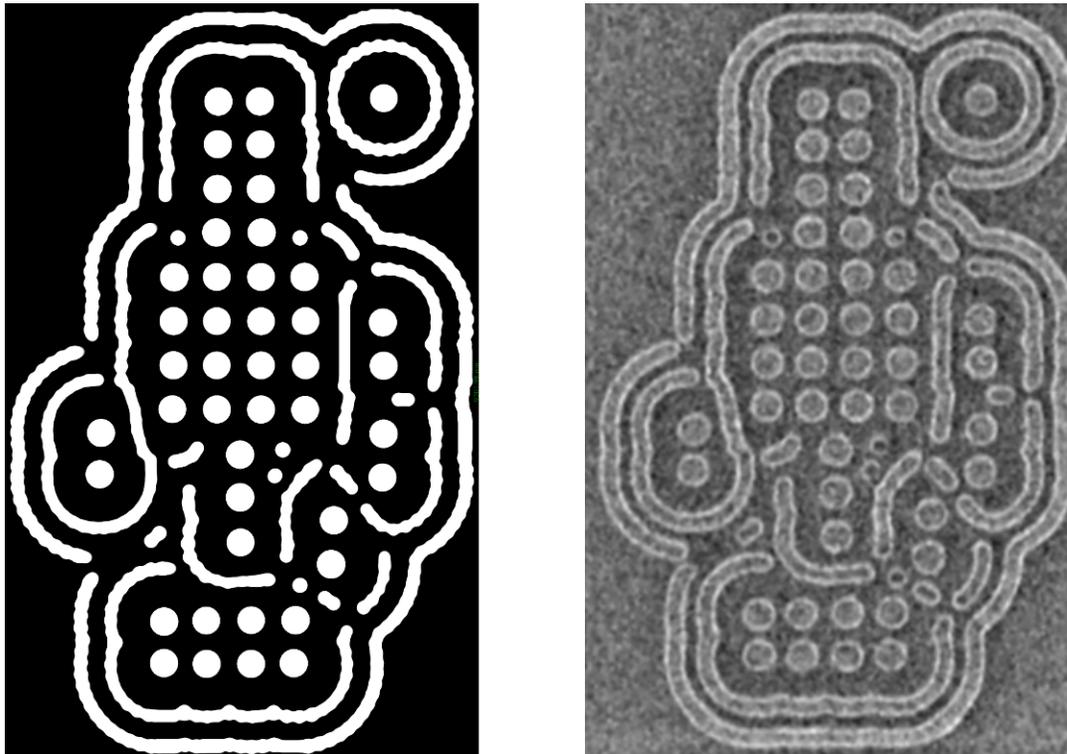
Figure 12. Simulated e-beam mask image (left) and resist exposed pre-etch SEM picture (right) of the ideal ILT mask shown in Figure 9. The contact mask diameter is 320 nm and the SRAFs are around 150 nm.
