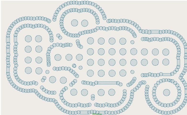
Figure 11. MB-MDP results using overlapping circular e-beam shots for a 22 nm random logic contact layout achieves a 22% reduction in shot count compared to the conventionally fractured Manhattanized mask shown in Figure 10.
