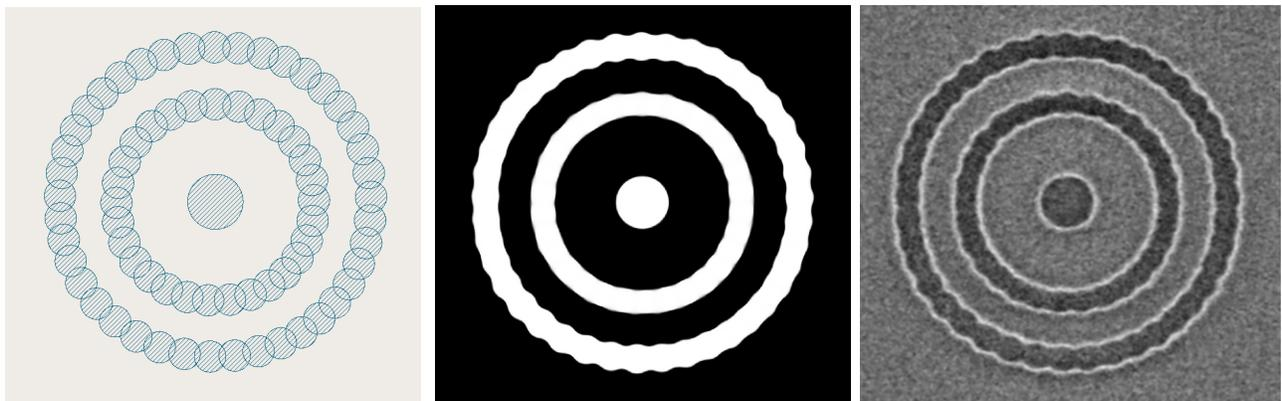
Figure 6. MB-MDP results for 1000 nm pitch contacts (pattern C0-4) using overlapping circular shots (left), simulated e-beam mask image (center), and the corresponding mask SEM image (right).
