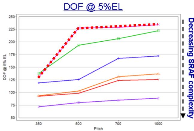
Figure 7. Depth of Focus (DOF) at 5% exposure latitude for contact pitches of 350 nm to 1000 nm and decreasing complexity of sub-resolution assist features (SRAFs) from top to bottom. The patterns used in this study have the most complex SRAFs (red dashed line).
