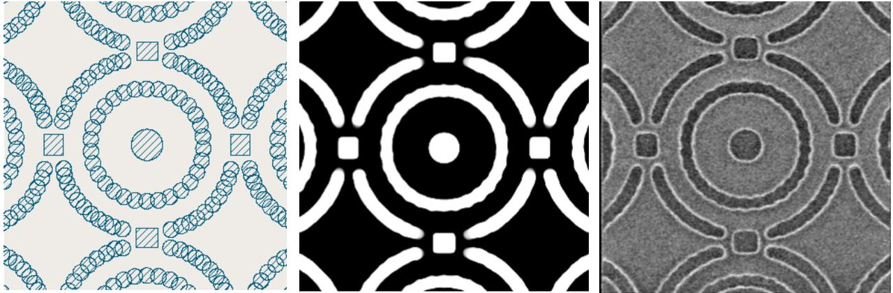
Figure 4. MB-MDP results for 500 nm pitch contacts (pattern C0-2) using overlapping circular shots (left), simulated e-beam mask image (center), and the corresponding mask SEM image (right).
