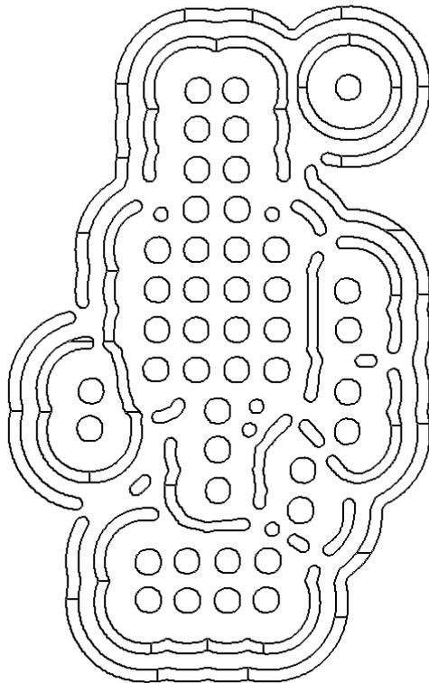
Figure 9. Ideal ILT mask of a random logic contact layout using Inverse Synthesizer™.
