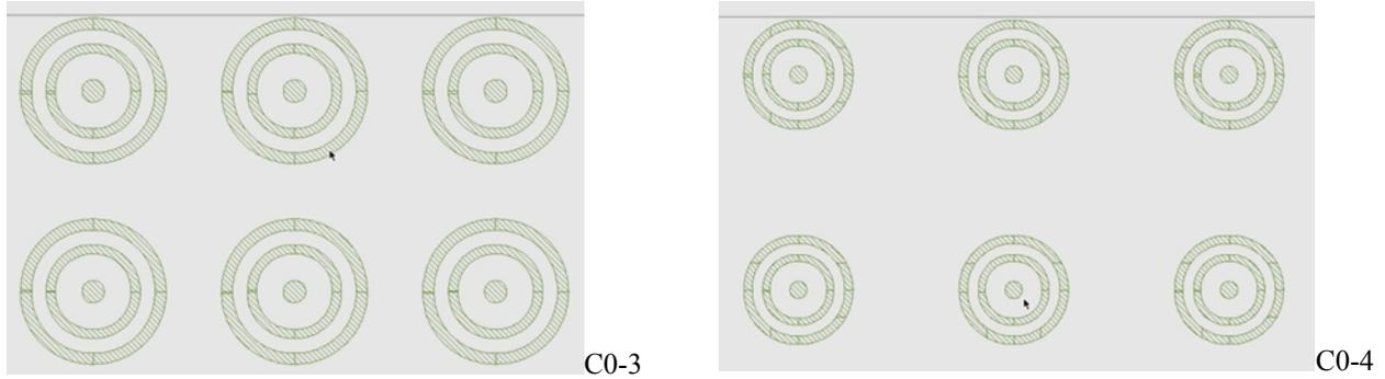
Figure 2. Differently spaced isolated contacts with ideal, curvilinear ILT patterns. In wafer dimensions the contact pitches are 350 nm, 500 nm, 700 nm and 1000 nm for the patterns C0-1 through C0-4, respectively.
