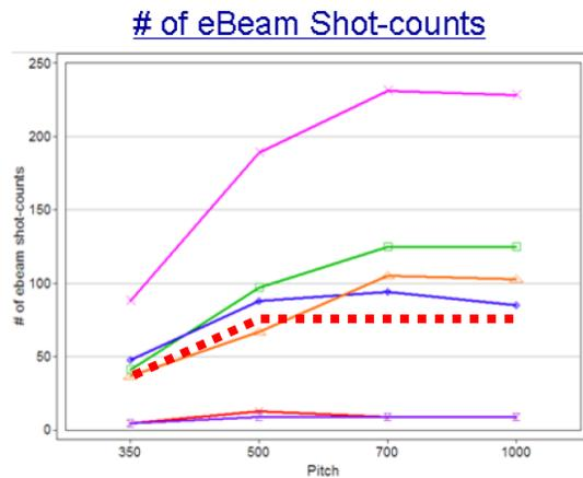
Figure 8. E-beam shot count vs. contact pitch and decreasing SRAF complexity from top to bottom. While the top line shows the conventional shot count for the most complex SRAFs the red dashed line shows the largely reduce shot count for the same SRAFs achieved with MB-MDP.
