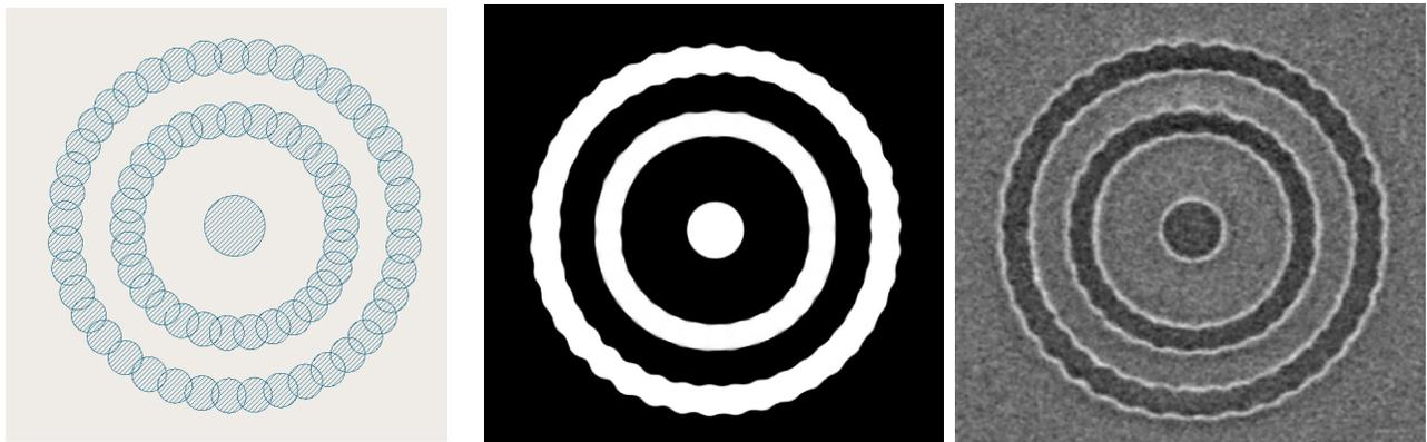
Figure 5. MB-MDP results for 700 nm pitch contacts (pattern C0-3) using overlapping circular shots (left), simulated e-beam mask image (center), and the corresponding mask SEM image (right).
