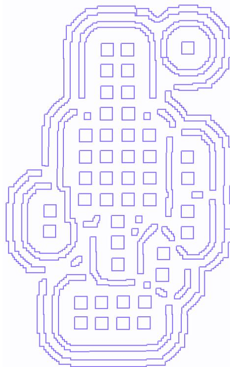
Figure 10. Optimized Manhattan version of an ILT mask for the same contact layout shown on the left.
