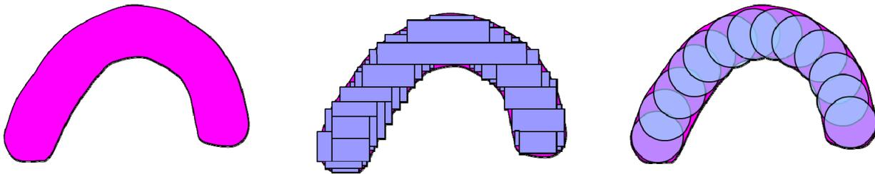
Figure 1. Comparison of conventional type fracturing (center) with MB-MDP using overlapping circles (right) for an ILT-type target shape (left).
