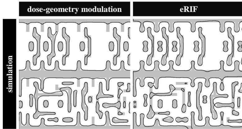
Figure 5. The evaluation of PEC by dose-geometry modulation and eRIF through the simulation of actual SRAM metal 1 layer with the designed CD of 25nm. The identical PSF parameters of nCAR and the area of simulation,  $1 \times 1 \mu\text{m}^2$ , were practiced for both modulations. The light grey areas demonstrate the designed layout and the exposed profile of resist overlapped on top of it as thick contours.
