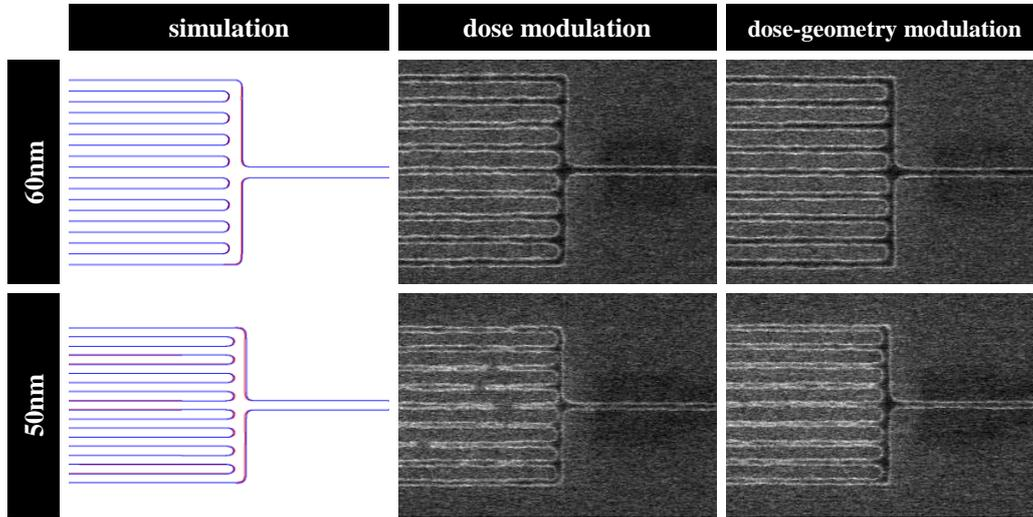
Figure 1. Comparison of the conventional dose modulation and dose-geometry modulation in the real test exposed images along with that of simulation results. The red contour corresponds the result obtained from the dose modulated correction and the blue one depicts the outcome of dose-geometry modulated correction in the simulation. All cases, simulations and test exposures, applied with same PSF parameters of nCAR for the direct comparisons.
