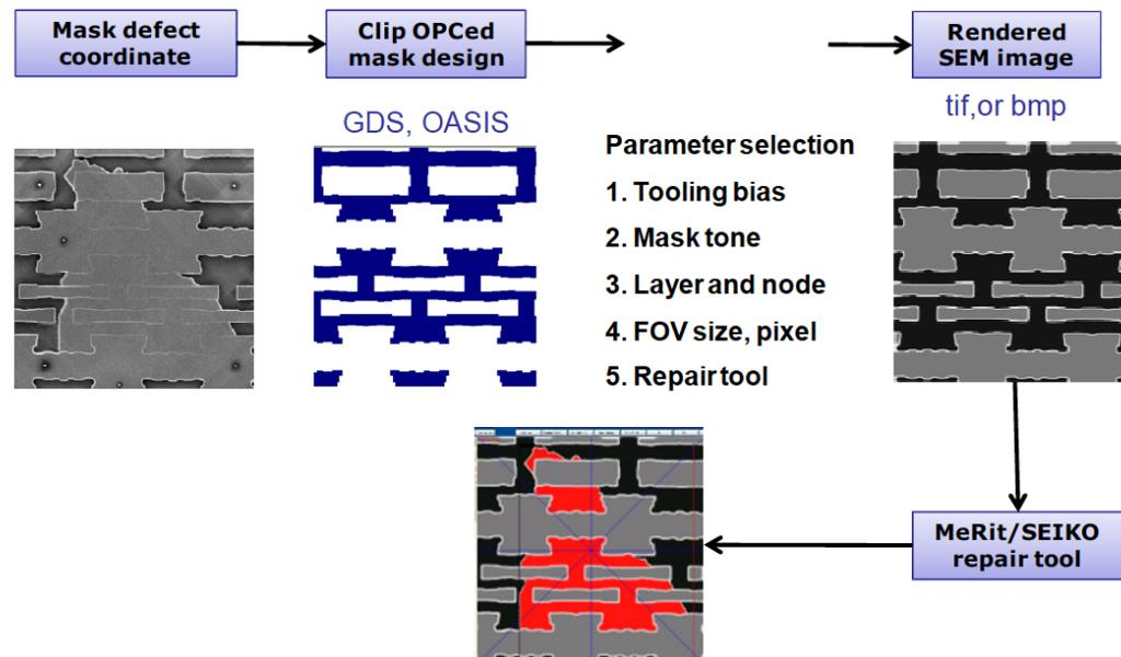
Figure 21. LAIPH Reference Pattern Generator (RPG) for mask repair flow
