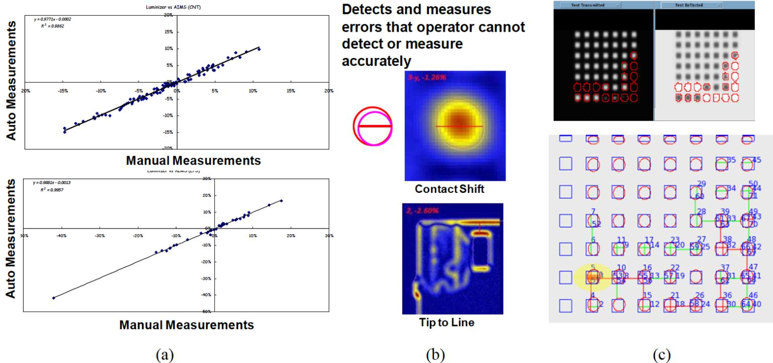
Detects and measures errors that operator cannot detect or measure accurately
