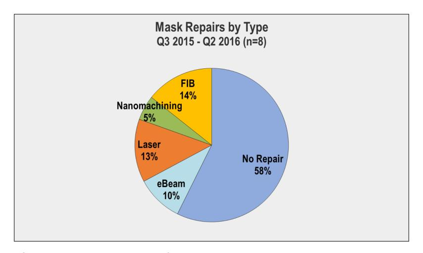
Q: What was the percentage of masks repaired by...no repair, eBeam, laser, nanomachining, FIB?
