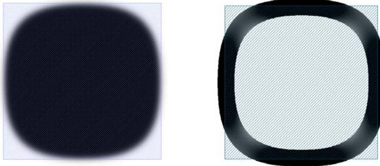
Figure 3. Simulated contour of a 100 nm x 100 nm VSB shot (left) and the corresponding edge slope showing larger than 1.7% dose change per 1 nm slope in black and lower than 1.4% dose change per 1 nm slope in white (right).
