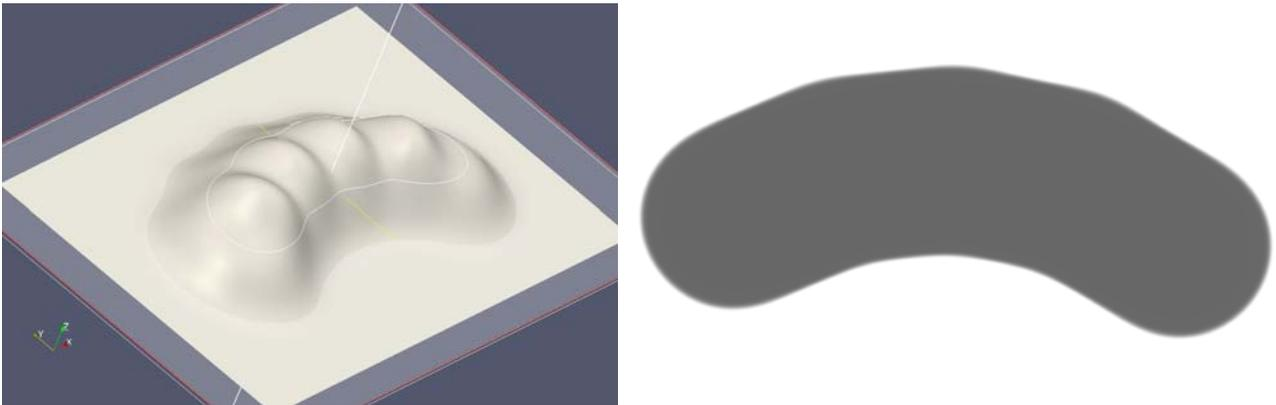
Figure 2. 3D dose map plot of the shapes shown in Figure 1 (left). Contour at 0.5 resist threshold (right).
