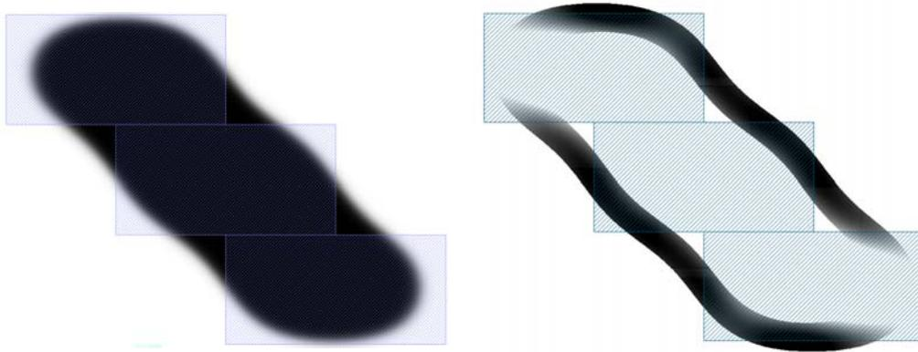
Figure 6. Simulated contour of 3 stacked 90 nm x 45 nm VSB shots shifted horizontally by 45 nm (left) and the corresponding edge slope showing larger than 1.7% dose change per 1 nm slope in black and lower than 1.4% dose change per 1 nm slope in white (right).
