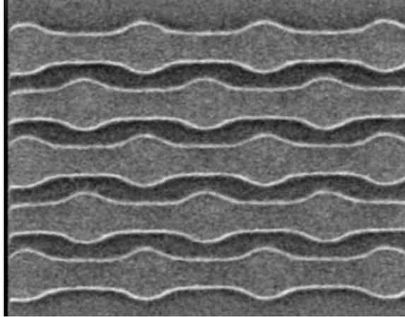
Figure 14. SEM image of the conventionally fractured wavy lines shown in Figure 12.
