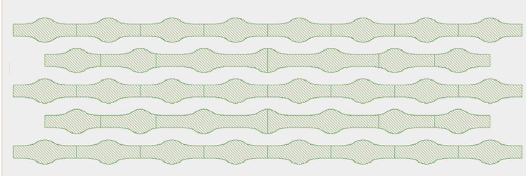
Figure 12. Desired mask shape of wavy metal 1 wires.
