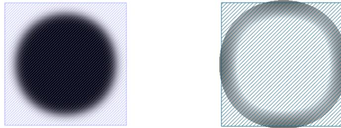
Figure 4. Simulated contour of a 60 nm x 60 nm VSB shot (left) and the corresponding edge slope showing larger than 1.7% dose change per 1 nm slope in black and lower than 1.4% dose change per 1 nm slope in white (right).
