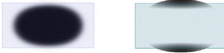
Figure 5. Simulated contour of a 90 nm x 45 nm VSB shot (left) and the corresponding edge slope showing larger than 1.7% dose change per 1 nm slope in black and lower than 1.4% dose change per 1 nm slope in white (right).
