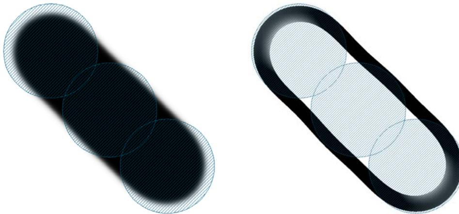
Figure 7. Simulated contour of circular shots of 72 nm diameter producing a similar mask shape as the 3 stacked VSB shots shown in Figure 6 (left) and the corresponding edge slope showing larger than 1.7% dose change per 1 nm slope in black and lower than 1.4% dose change per 1 nm slope in white (right).
