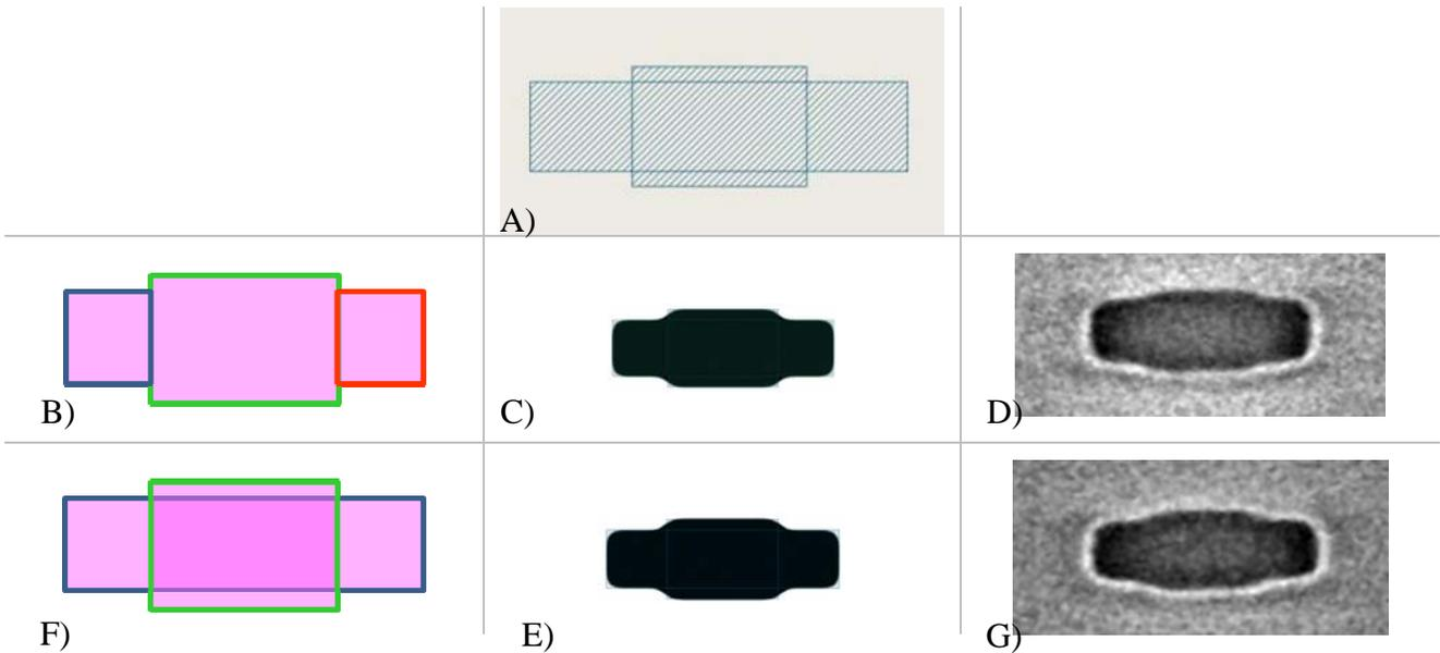
Figure 9. Comparison of a “wavy” line fractured conventionally or with MB-MDP. While the conventional method needs 3 shots for this example, the new method needs only 2 shots. Since the overlapping shot uses less than the full dose the mask write time for the new method is even shorter than 2/3 of the conventional method.
