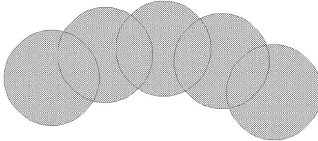
Figure 1. Overlapping circular e-beam shots each written with a dose amount of 1.0 so that the overlapping area receives a dose amount of 2.0.
