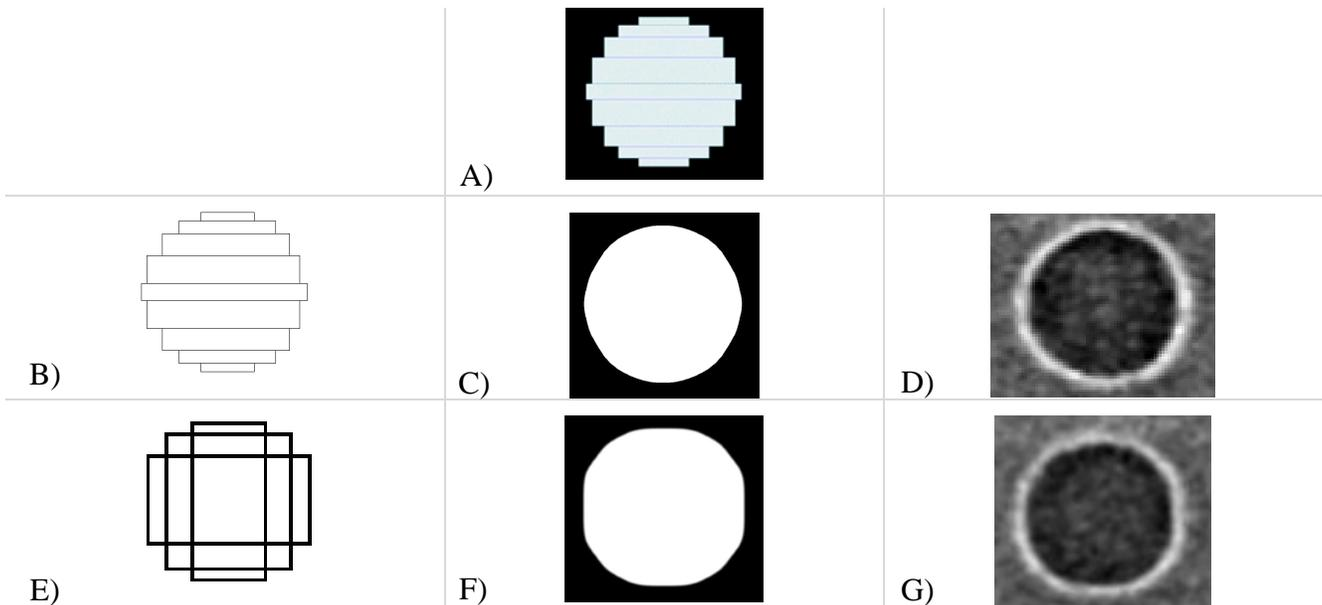
Figure 11. Comparison of a 308 nm diameter (mask dimensions) 3-step staircase contact/via fractured conventionally or with MB-MDP. While the conventional method needs 9 shots for this example, the new method needs only 3 shots.
