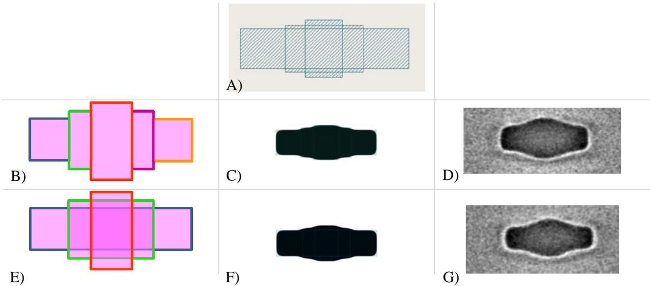
Figure 10. Comparison of a 3-step staircase line fractured conventionally or with MB-MDP. While the conventional method needs 5 shots for this example, the new method needs only 3 shots. Since the overlapping shots use less than the full dose the mask write time for the new method is only about half of the conventional method.
