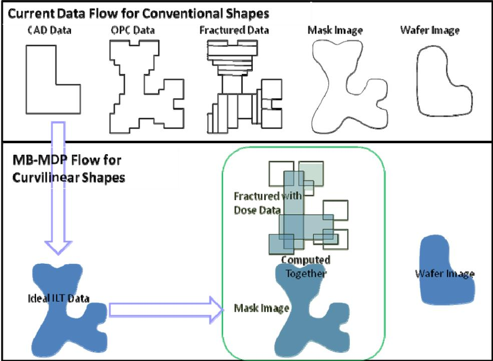
Figure 8. The Model Based Mask Data Preparation (MB-MDP) included in the conventional fracturing flow where MB-MDP processes curvilinear shapes while rectangular shapes are fractured conventionally.
