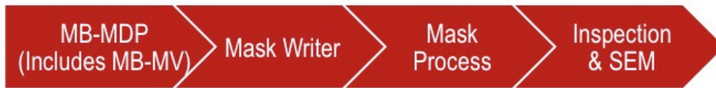
Figure 3. For those mask shops that employ MB-MDP, MB-MV can be completed before mask writing to maximize time and resource savings.
