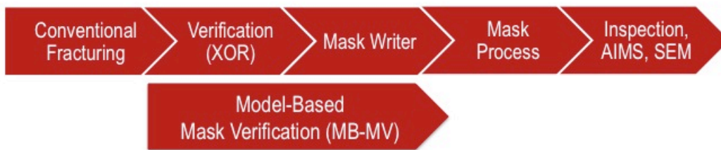
Figure 4: MB-MV can be added to the current mask-inspection flow as a parallel process without introducing any new risk to the existing flow where a change to the flow is considered unacceptable.
