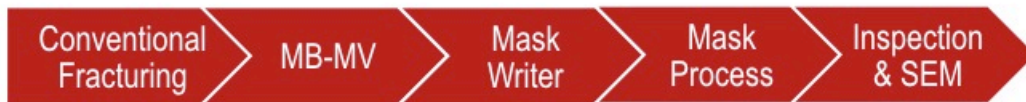
Figure 5. In some situations, mask shops may choose to insert MB-MV as a new step in the mask-making flow prior to mask writing.
